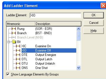
Figure 41: Adding an XIO Element
