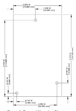
Figure 2: External Mounting Diagram
