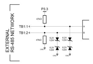
Figure 1: RS-485 Interface Circuitry Schematic
