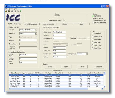
Figure 9: Configuration File Loaded
