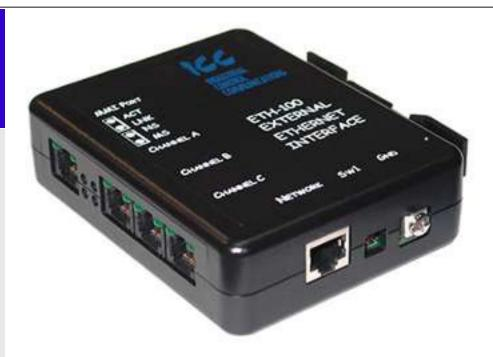
The ETH-100 provides ethernet connectivity to up to three Toshiba 7-series, 9-series or VF-nC1 Adjustable Speed Drives (ASDs) with Modbus TCP/IP, release 1.0 (Conformance class 0 and partial class 1 and class 2 compliant).
