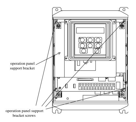
Figure 1: Elll with front cover removed
