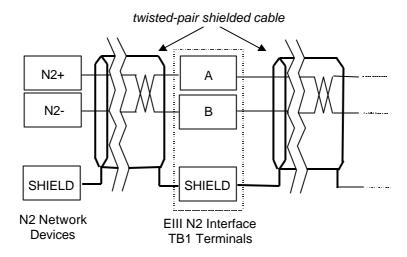
Figure 4. N2 Bus Cable Connection
