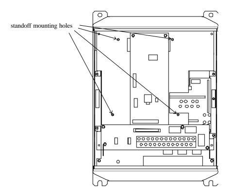
Figure 2: EllI with front cover and operation panel support bracket removed
