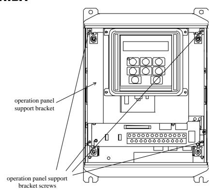
Figure 3: Elll with front cover removed
