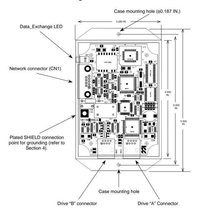
Note that the above diagram shows the PBDP-100 with its cover removed. However, it is not necessary to remove the cover in order to install or configure the PBDP-100.
